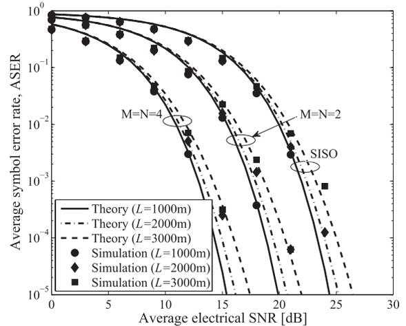
**Fig. 3** ASER versus average SNR,  $\bar{\gamma}$ , of SISO/FSO system,  $2 \times 2$  and  $4 \times 4$  MIMO/FSO systems using  $8 \times 4$  SC-QAM for various values of  $L$  with  $C_n^2 = 1 \times 10^{-15} \text{ m}^{-2/3}$ .
