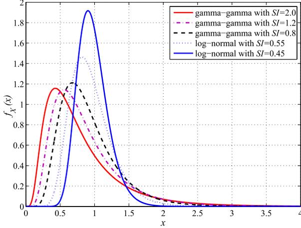
**Fig. 2** pdfs of different log-normal and gamma-gamma intensity distributions.
