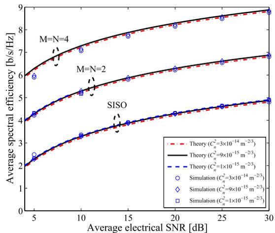
**Fig. 7** ASE,  $\bar{C}/B$ , versus the average electrical SNR,  $\bar{\gamma}$ , of different MIMO/FSO channels for different values of  $C_n^2$  with free-space link distance  $L = 1,000$  m.
