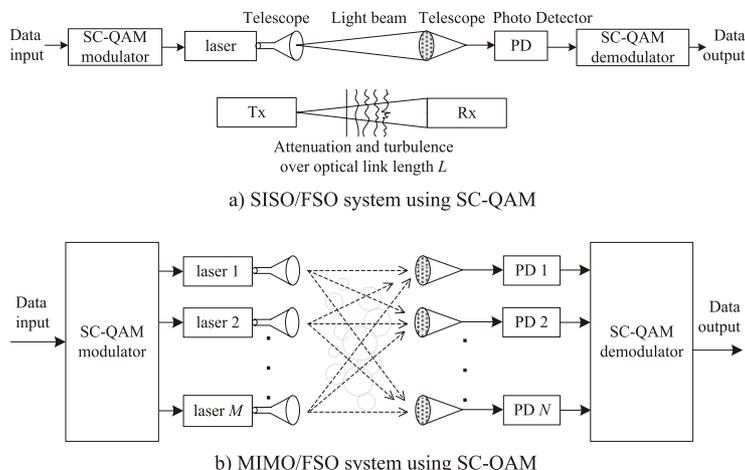
**Fig. 1** Block diagram of SISO/FSO and  $M \times N$  MIMO/FSO systems using SC-QAM signaling over atmospheric turbulence channel.
