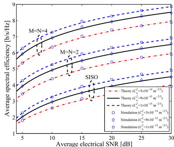
**Fig. 9** ASE,  $\bar{C}/B$ , versus the average electrical SNR,  $\bar{\gamma}$ , of different MIMO/FSO channels for different values of  $C_n^2$  with free-space link distance  $L = 6,000$  m.
