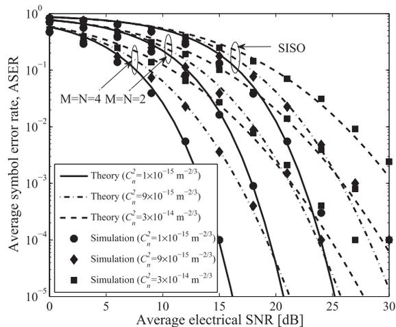
**Fig. 4** ASER versus the average SNR,  $\bar{\gamma}$ , of SISO/FSO system,  $2 \times 2$  and  $4 \times 4$  MIMO/FSO systems using  $8 \times 4$  SC-QAM for various values of  $C_n^2$  for weak, moderate, and strong atmospheric turbulence conditions with free-space link distance of  $L = 2,000$  m.
