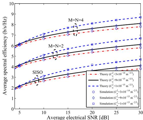
**Fig. 8** ASE,  $\bar{C}/B$ , versus the average electrical SNR,  $\bar{\gamma}$ , of different MIMO/FSO channels for different values of  $C_n^2$  with free-space link distance  $L = 3,000$  m.
