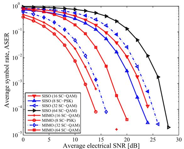
**Fig. 6** ASER versus the average SNR,  $\bar{\gamma}$ , of SISO/FSO and  $4 \times 4$  MIMO/FSO systems with different QAM multiplicities;  $C_n^2 = 1 \times 10^{-15} \text{ m}^{-2/3}$ , and free-space link distance  $L = 2,000$  m.
