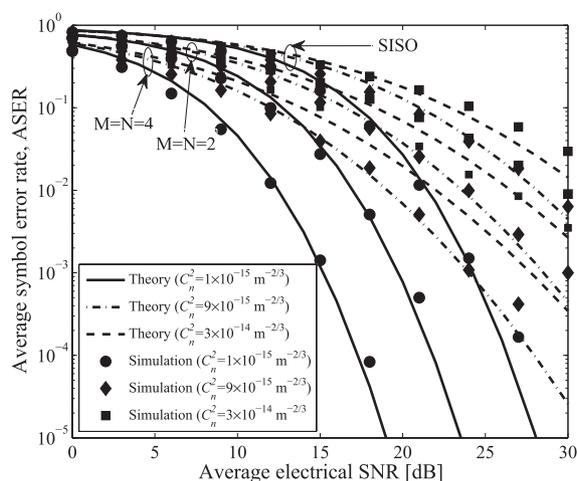
**Fig. 5** ASER versus the average SNR,  $\bar{\gamma}$ , of SISO/FSO system,  $2 \times 2$  and  $4 \times 4$  MIMO/FSO systems using  $8 \times 4$  SC-QAM for various values of  $C_n^2$  for weak, moderate, and strong atmospheric turbulence conditions with free-space link distance  $L = 4,000$  m.
