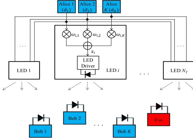
Fig. 1: MU-MISO VLC system with  $N_T$  LED arrays for  $K$  non-cooperative legitimate pairs of user (Alice and Bob) with mutual confidentiality, and one Eavesdropper (Eve).
