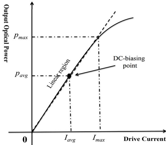
Fig. 2: Nonlinear LED transfer characteristic.
