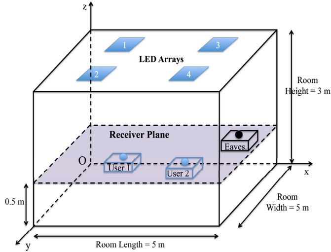
Fig. 4: Geometrical configuration of MU-MISO VLC wiretap channel.
