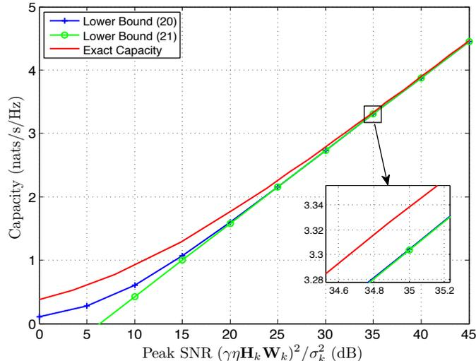
Fig. 3: Exact and lower bounds capacity of amplitude-constrained scalar Gaussian channels.
