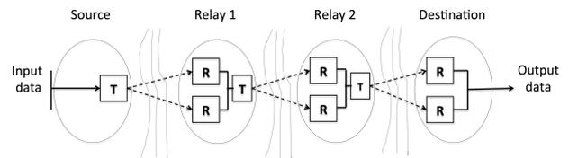
**Fig. 1** Multihop SIMO system with two relay nodes and two receive apertures at each node.
