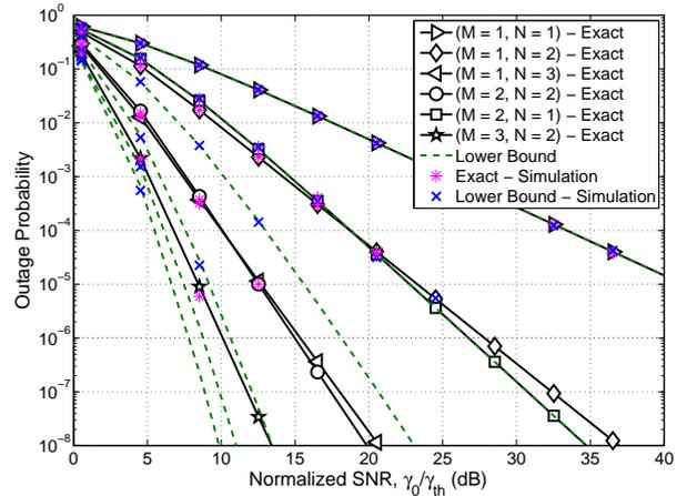
**Fig. 9** AF relaying: Outage probability versus normalized SNR for independent fading with different numbers of hops and receive apertures,  $C_n^2 = 5 \times 10^{-15}$ ,  $L = 8000$  m.
