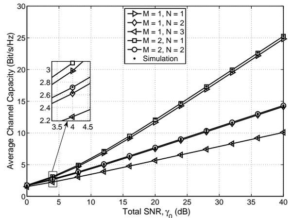
**Fig. 12** DF relaying: Average channel capacity versus total SNR for correlated fading  $\rho = 0.5$  with different numbers of hops and receive apertures,  $C_n^2 = 10^{-14}$ ,  $L = 8000$  m.
