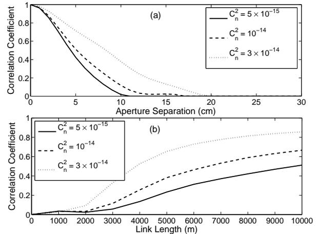
**Fig. 2** (a) Correlation coefficient versus aperture separation for different values of turbulence strength and link range  $L = 4000$  m; (b) Correlation coefficient versus link range for different values of turbulence strength and aperture separation  $d = 8$  cm.
