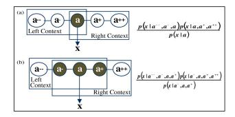
Figure 1: Bayesian pentaphone model composition. (a) is composed of the preceding/following triphone-context unit and center-monophone unit and (b) is composed of the preceding/following tetraphone-context unit and center-triphone-context unit.
