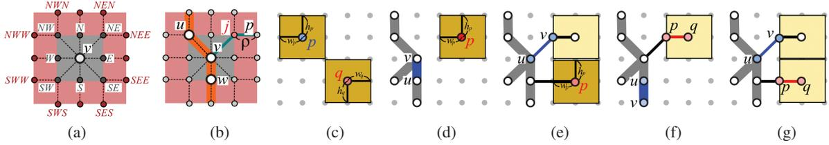
**Figure 5:** Aesthetic constraints for spatially-efficient map design. (a) Twelve leader styles. (b) Aligning a leader line to make a maximal angle with adjacent metro lines. Checking overlap between (c) two labels, (d) a label and a metro line segment, (e) a label and a leader line segment, (f) leader and metro line segments, and (g) two leader line segments.
