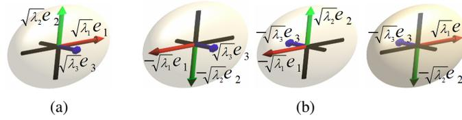
**Fig. 2.** Sign ambiguity of eigenvectors. (a) A tensor can be represented by an ellipsoid. The directions of the coordinate axes are represented by the arrows. Different colors are assigned to the axes for representing the magnitudes of eigenvalues. (b) Three other possible definitions of the tensor in (a).
