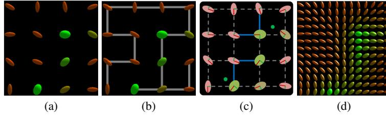
**Fig. 5.** MST-based clustering in tensor field: (a) Original tensor samples (b) The final MST that covers all the tensor samples. (c) Degenerate points (green points) and degenerate pairs (blue lines) obtained through the MST-based clustering algorithm. (d) Interpolated result obtained through the MST-based clustering algorithm only.
