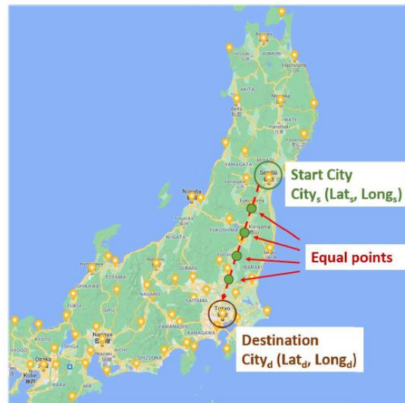
(b) An Example of Power Consumption Prediction for A Single Trip from Sendai to Tokyo in Japan. Each yellow star denotes a city associated with an explicit weather record. Created from Google Map [52].
