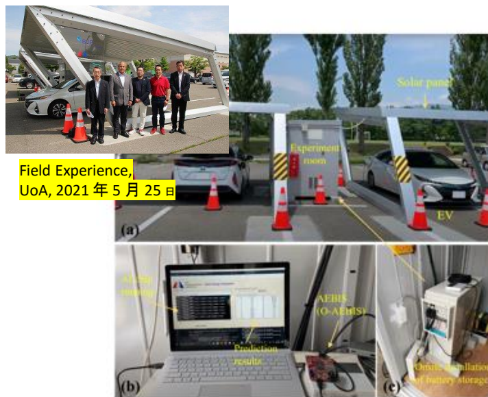
Fig. 5. A demonstration of the energy management system based on our system named AEBIS and its optimized version O-AEBIS.
